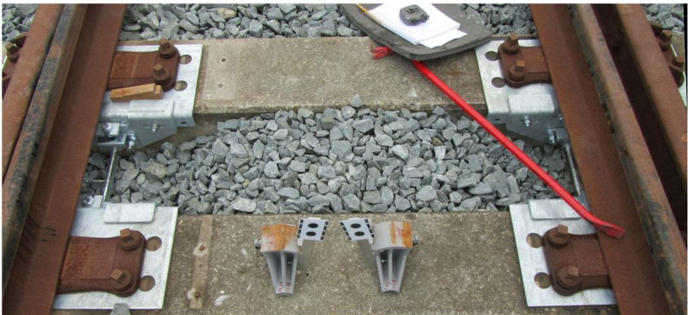
Figure 6 Disassembled blocks during inspection and measuring
