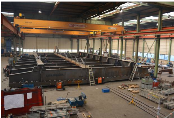
Figure 11. Production of steel deck
