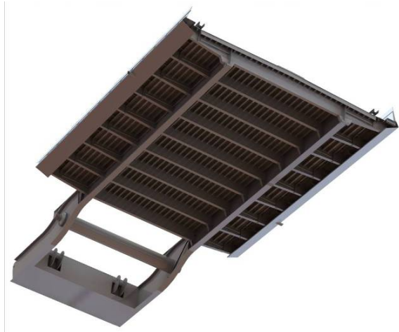
Figure 7. Steel deck in Inventor
